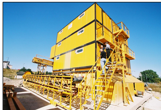
Figure E-11. Slurry Treatment Facilities (Stacked Configuration)
