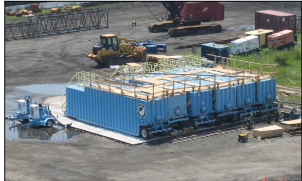
Figure E-10. Typical Slurry Mixing Plant
