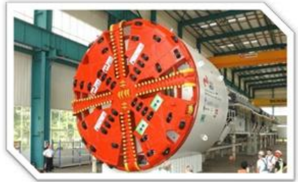
Figure E-5. Typical Pressurized-Face TBM
