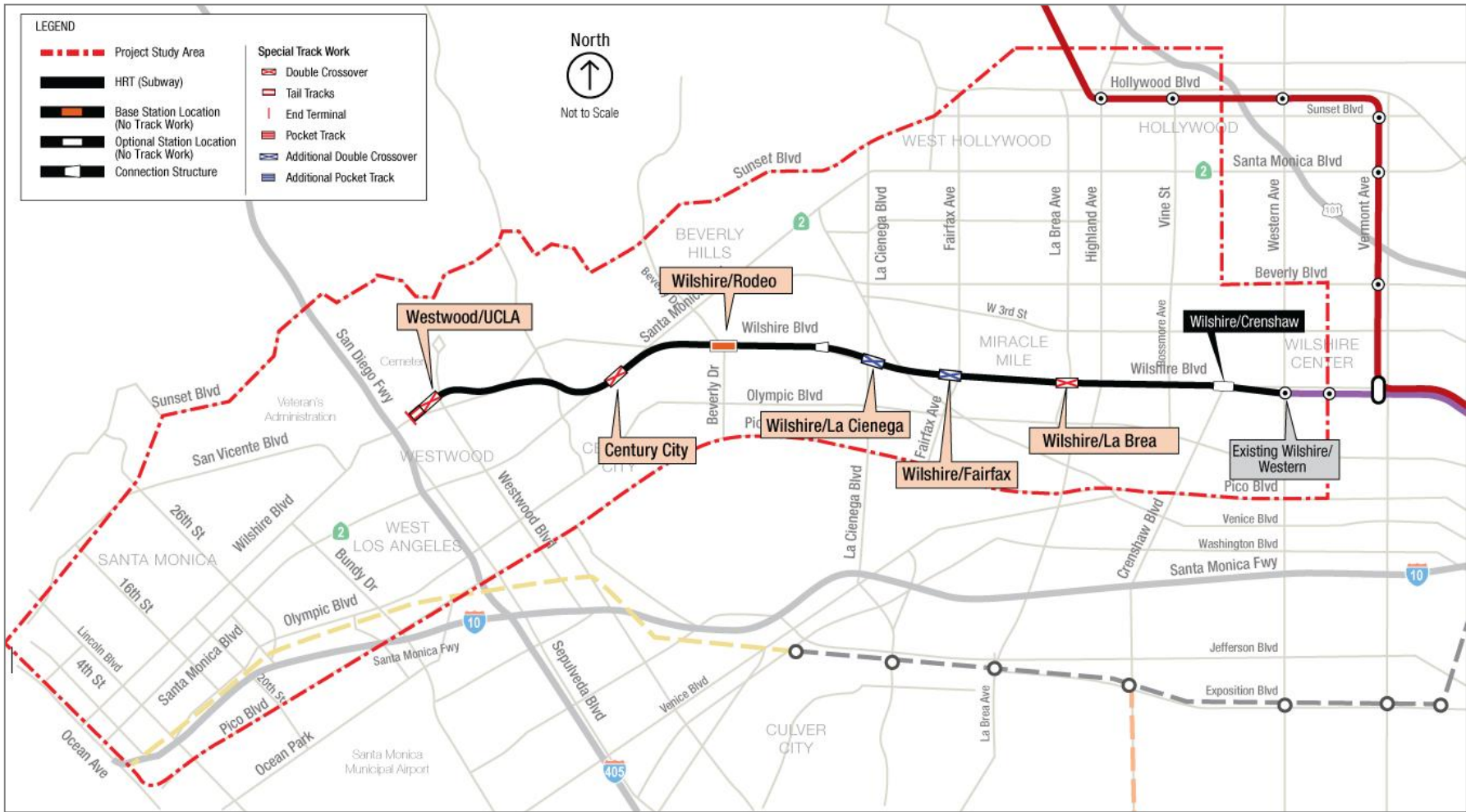
Figure 2-56. Special Trackwork Locations for Alternative 1
