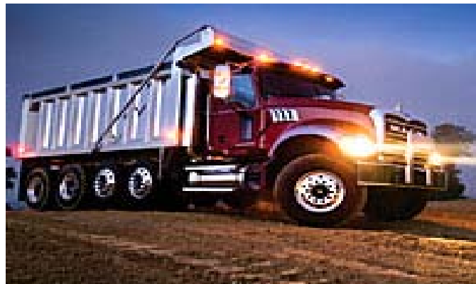
Figure 4-79. Haul Truck for Excavated Soil Removal with Cover Mechanism Shown
