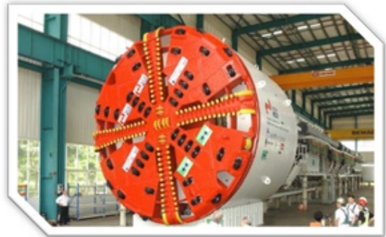
Figure 4-9: Typical Pressurized-Face TBM
