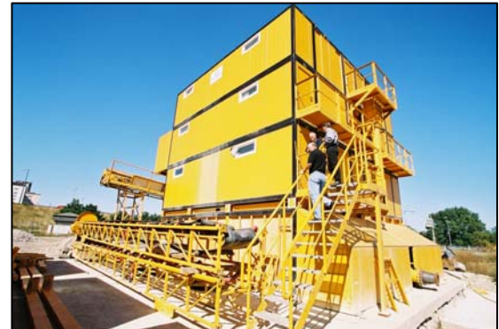
Figure 4-21: Typical Slurry Treatment Facilities (Stacked Configuration)
