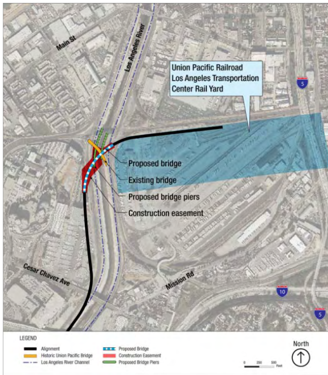
Figure 2-14. UP Railroad Rail Bridge
