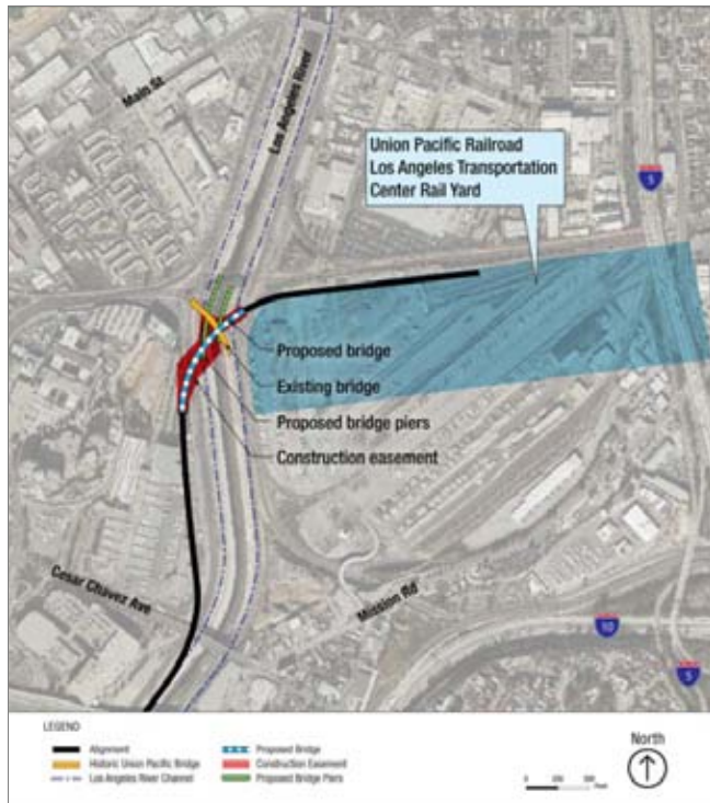
Figure 2-14. UP Railroad Rail Bridge
