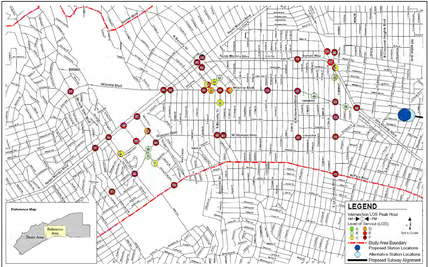
Figure 4-5. Year 2035 MOS 1 Intersection Levels of Service (continued)
