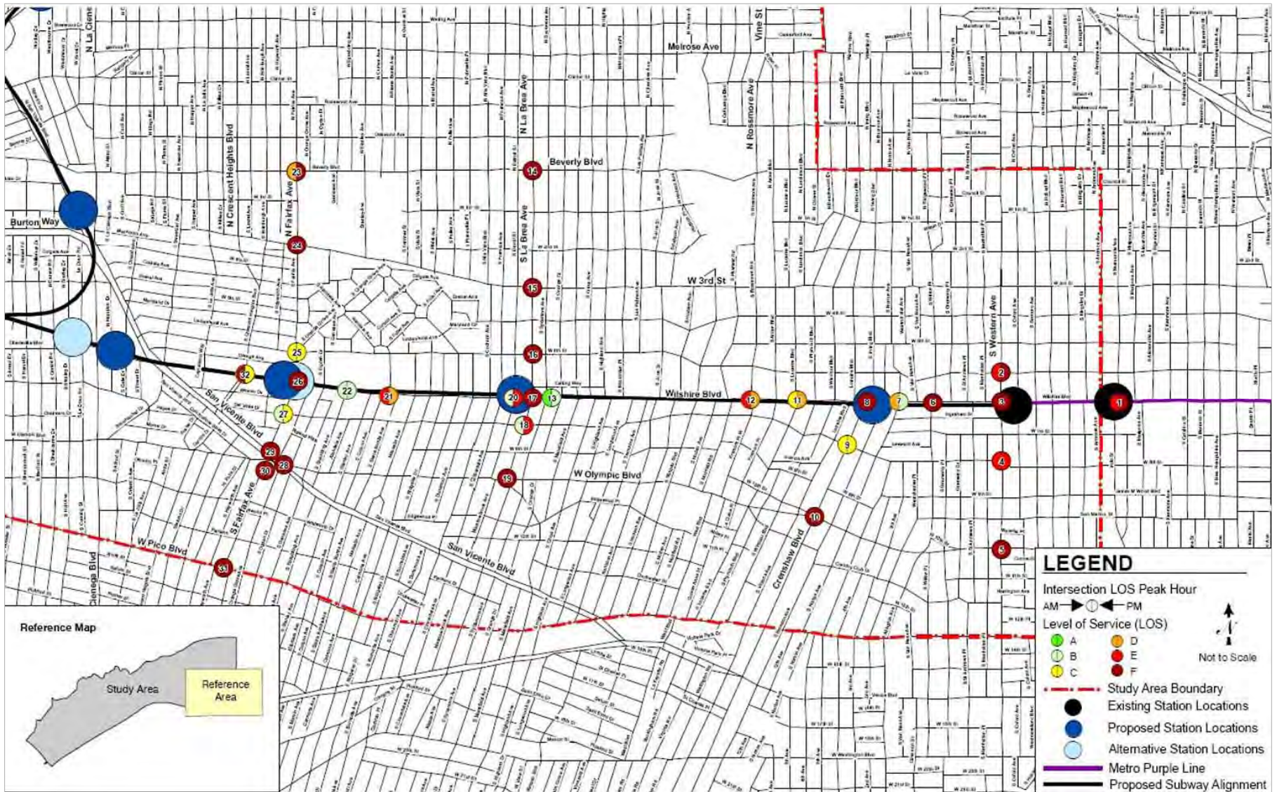
Figure 5-42. Year 2035 Alternative 4 Intersection Levels of Service
