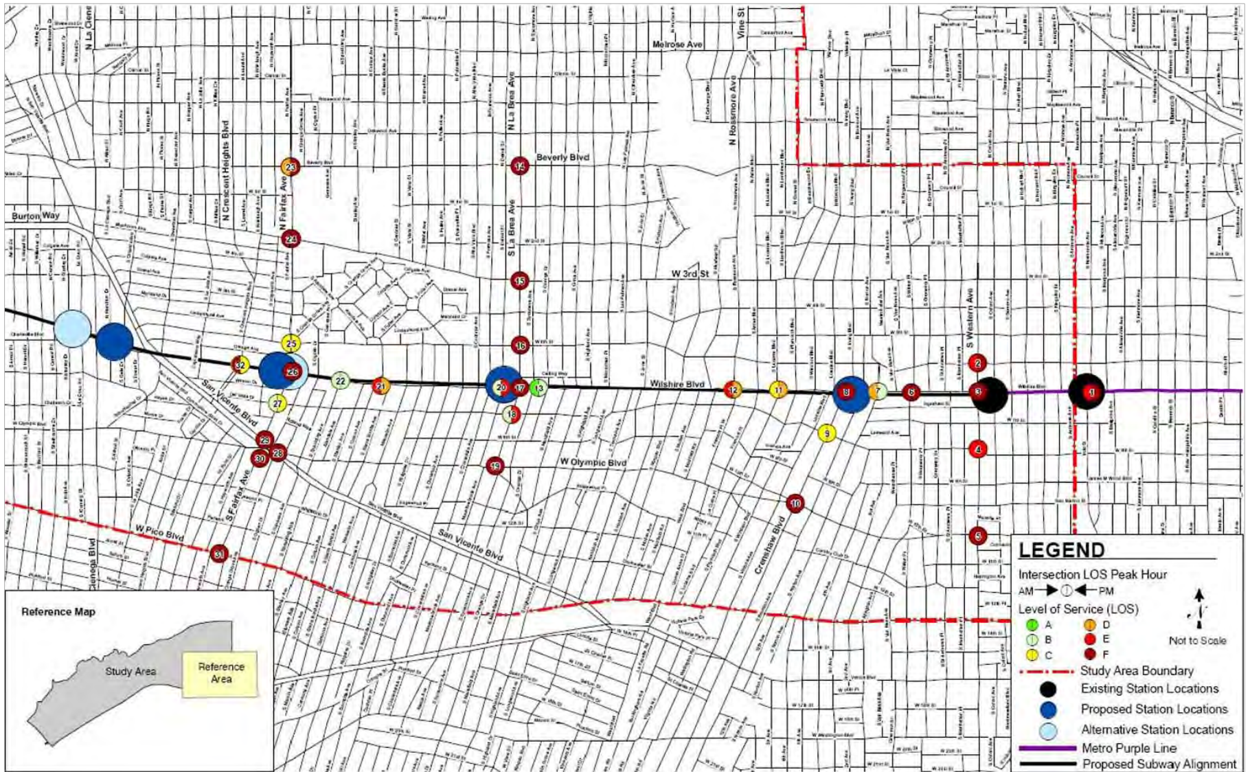
Figure 5-39. Year 2035 MOS 2 Intersection Levels of Service
