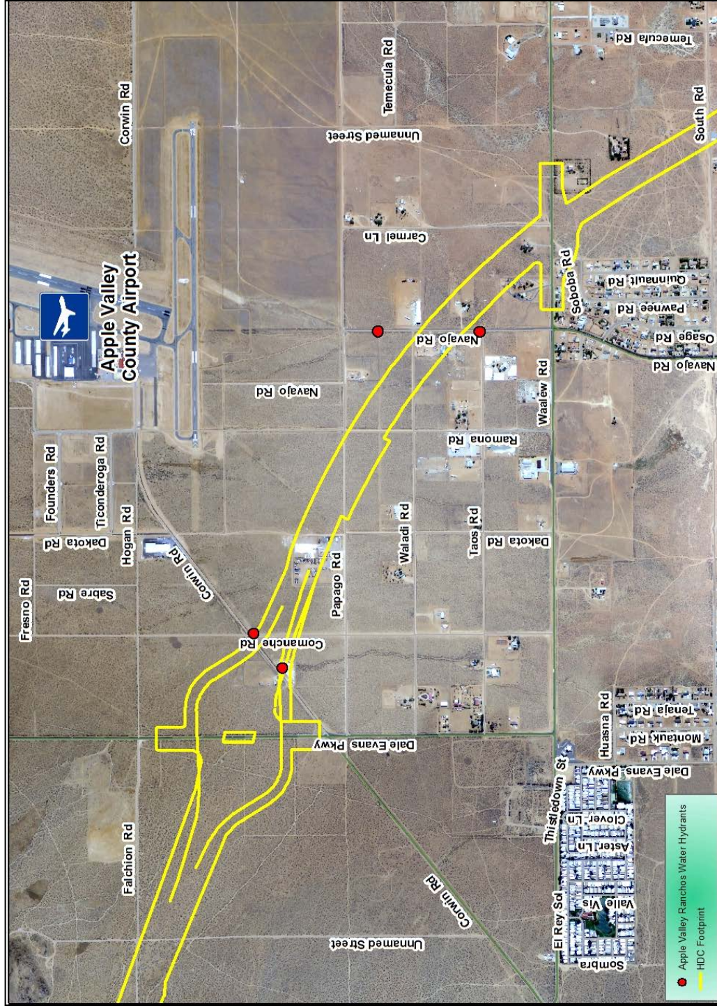
Figure 3.1.5-11 Fire Hydrant Locations in San Bernardino County Portion of the High Desert Corridor Project (Section 4)
