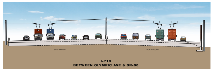
The Zero Emission Extension (ZEE) option under Alternatives 6B and 6C would extend zero emission technology all the way to SR-60.
