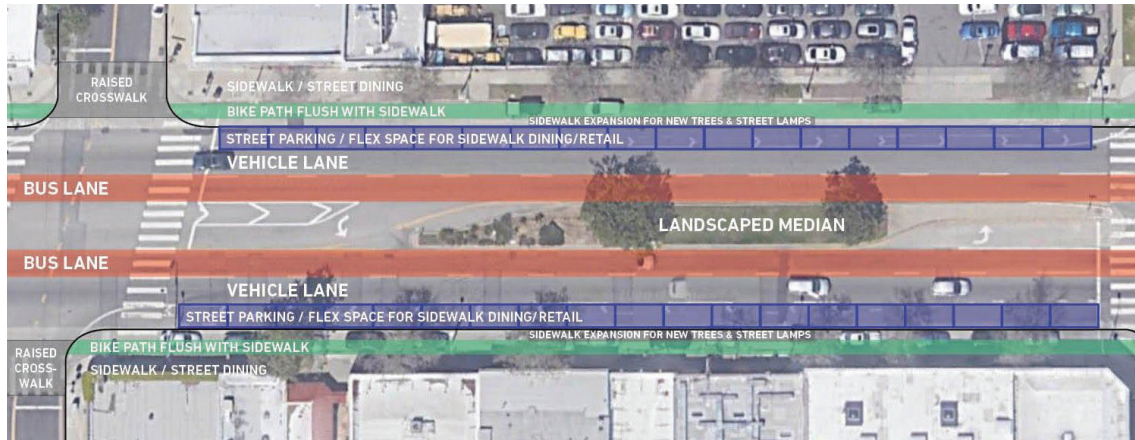
Proposed layout within Zone 2 showing expanded sidewalks, raised bike paths & crosswalks, maintained parking
