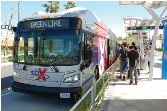
Example central station for left-side boarding
