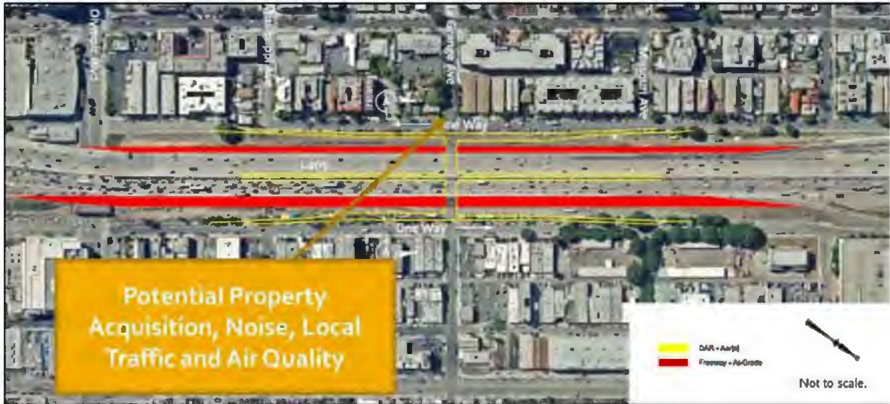
Figure 14b. Environmental Concerns at the La Grange Direct Access Ramp
