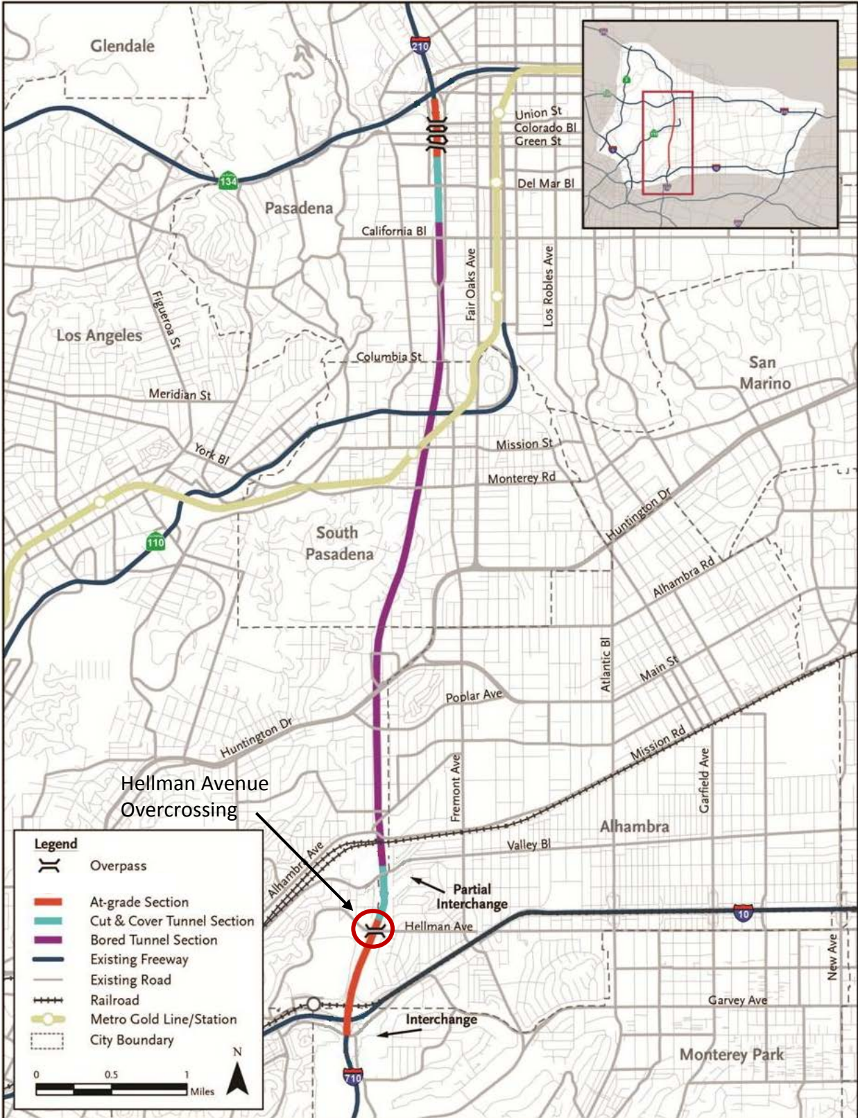
Project Vicinity Map State Route 710 North Study Freeway Tunnel Alternative Alignment Dual Bore Option
