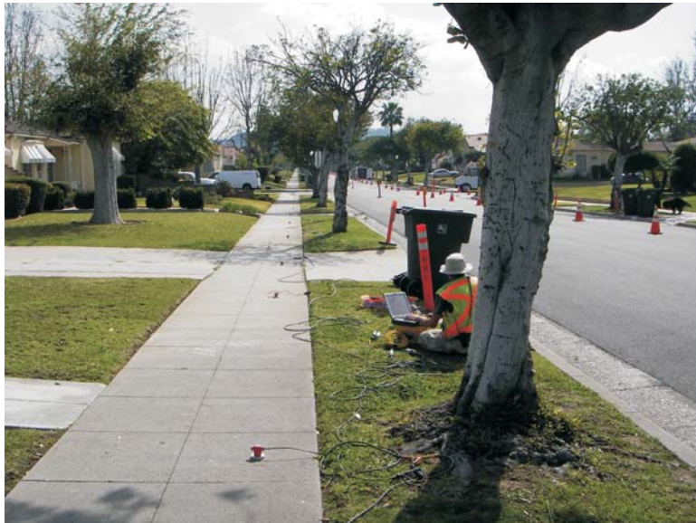
TYPICAL PASSIVE SURFACE WAVE SETUP
