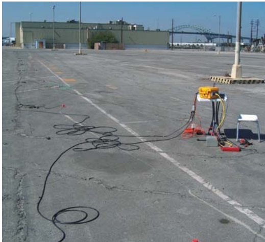
Refraction Microtremor Array Layout
