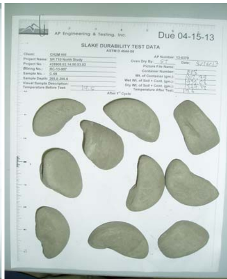
After First Cycle Type I: Pieces virtually unchanged.
