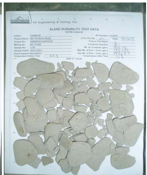
After Second Cycle Type II Large and Small Fragments
