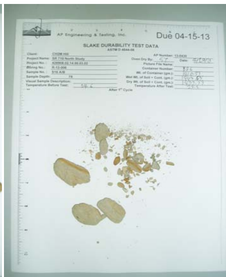
After First Cycle Type III Exclusively small fragments
