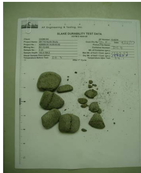
After First Cycle Type II Large and Small Fragments
