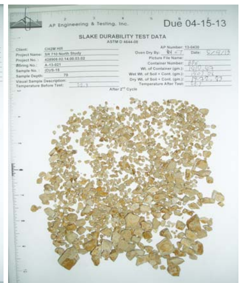
After Second Cycle Type III Exclusively small fragments
