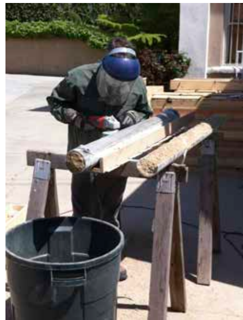
Figure 5. Cutting open the poly tubes used in the upper 100 feet of both sonic borings.
