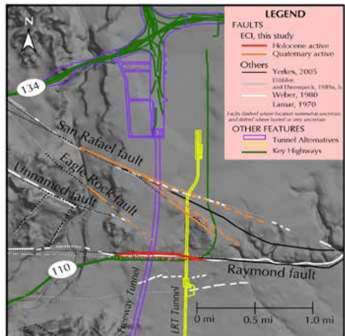
Figure 1. Map of the potentially active faults that may impact the proposed tunnel routes. There are different mapping interpretations and locations for San Rafael, Eagle Rock, and other northwest-trending faults, but in this discussion, they are collectively referred to as the Eagle Rock-San Rafael fault zone. An expanded version of this figure is included as Plate 1 in this TM.
