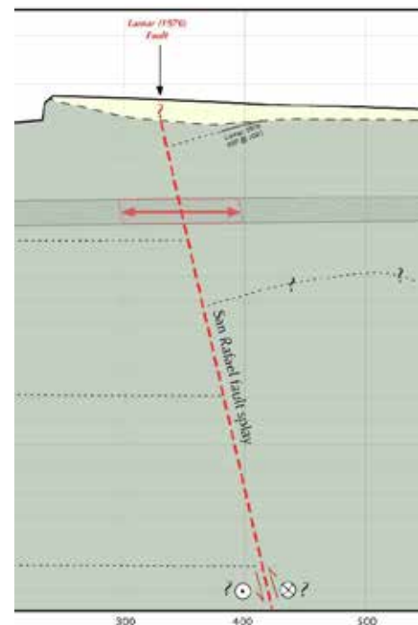
Figure 15. Interpreted additional secondary splay of the San Rafael fault that projected along strike to the LRT Alternative, shown in light gray shading. The fault location uncertainty zone is shown by red arrows across the tunnel section.
