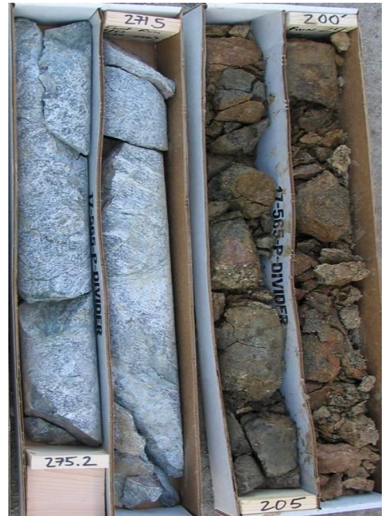
Exhibit 4-5. Basement Rocks. Igneous and metamorphic rocks from SR 710 North Study Area. The two cores on right are weathered rocks and the two cores on left are fresh rock.
