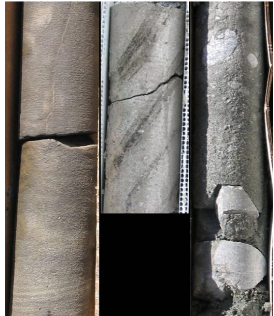
Exhibit 4-4. Topanga Formation. Core on right is conglomerate with sandstone matrix; core in middle is sandstone with siltstone laminations; core on left is siltstone/ mudstone.
