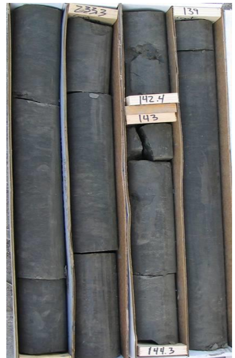
Exhibit 4-2. Fernando Formation. Core from SR 710 North Study Area, showing consistent nature of the unbedded Siltstone Member.
