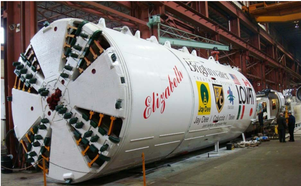
Figure 10. Brightwater TBM with Ripper-Style Cutting Tools for Soil or Soft Ground Conditions
