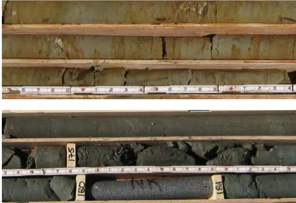
Figure 5: Typical Fernando Formation Core Samples (RMT Tf) (Cores from Boring RC-13-007)
