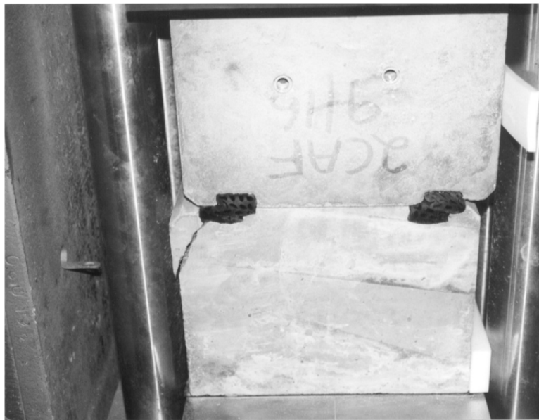
Figure 11. Segment Testing showing Tensile Splitting due to Gasket Compression (Swartz et al., 2002)
