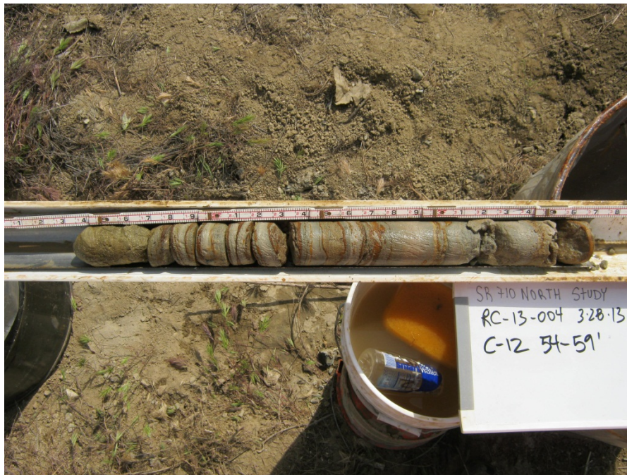
Figure 5: Boring RC-13-004 Core (Puente Formation) from 54 to 59 feet below grade
