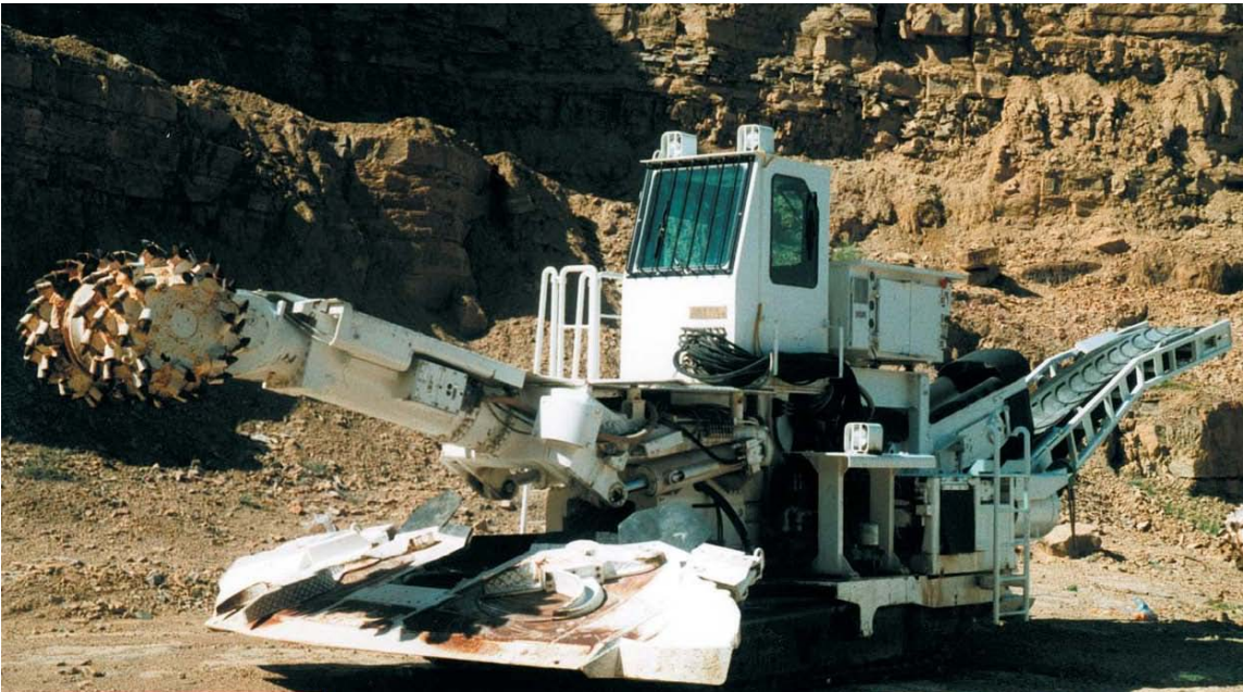
Figure 14. A 50-ton Class Roadheader Layout
