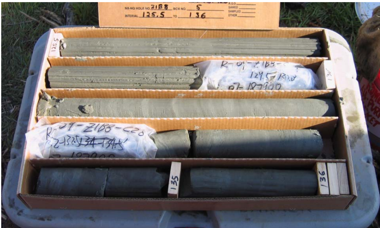
Figure 3: Boring Z1-B8 Core (Puente Formation) from 125 to 135 feet below Grade
