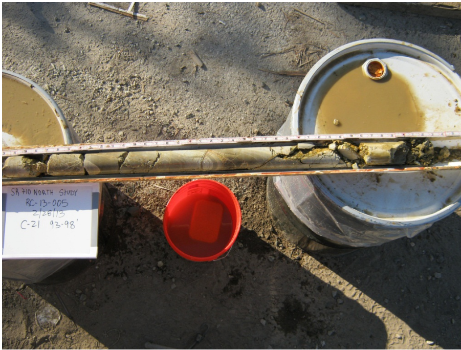
Figure 4: Boring RC-13-005 Core (Puente Formation) from 93 to 98 feet below grade
