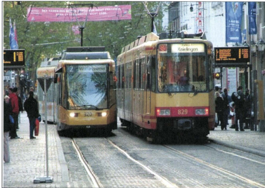
Exhibit 7. Example of Streetcar and LRT (Modern Streetcar on Left, LRT on Right)
