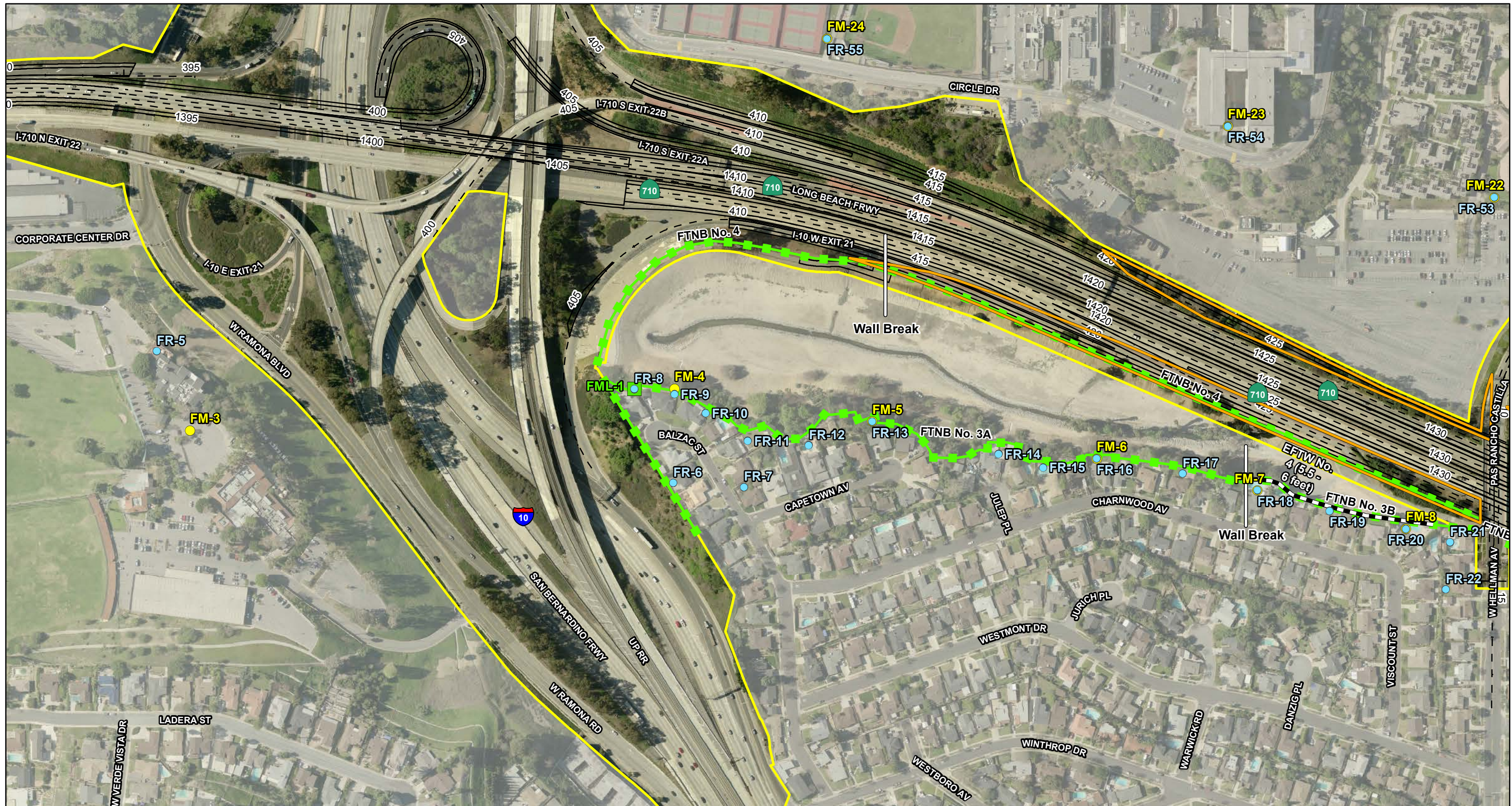
FIGURE 3.14-7 Sheet 3 of 15 SR 710 North Project Noise Measurement and Receptor Locations and Modeled Noise Barriers - Freeway Tunnel Alternative Dual Bore Design 07-LA-710 (SR 710) EA 187900 EFIS 0700000191
