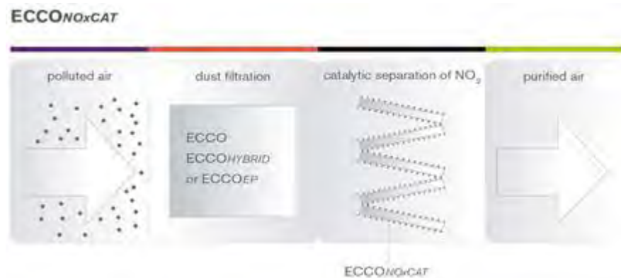
Schematic drawing of the ECCONoxCAT filter (source: www.aigner.at )
