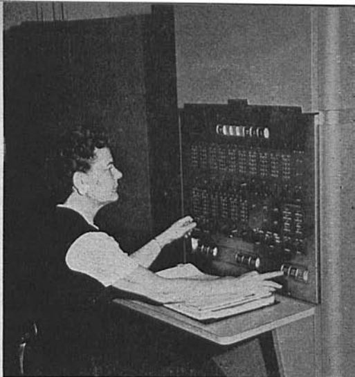
THE "650" DATA PROCESSOR , our newest, is a lightning fast computer with a "memory." From her operating manual, Helene Bates is setting the controls on the console unit for a calculator operation. In this console is the computer. At left is the power unit, which transforms building current into high-voltage direct current for use in electronic circuits. (See also photo on next page.)
