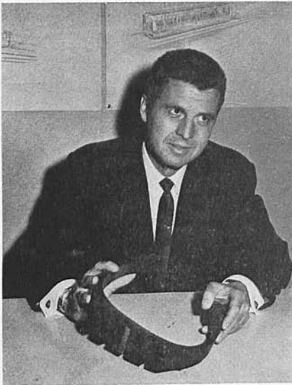
INSPECTING a section of rubber tire of special type planned for use on the supporting drive wheels of the proposed rapid transit cars is Irvan F. Mendenhall, President, Daniel, Mann, Johnson, & Mendenhall. Tire section contains a steel mesh fabric. On wall behind Mr. Mendenhall is concept of the rapid transit car proposed for MTA.
