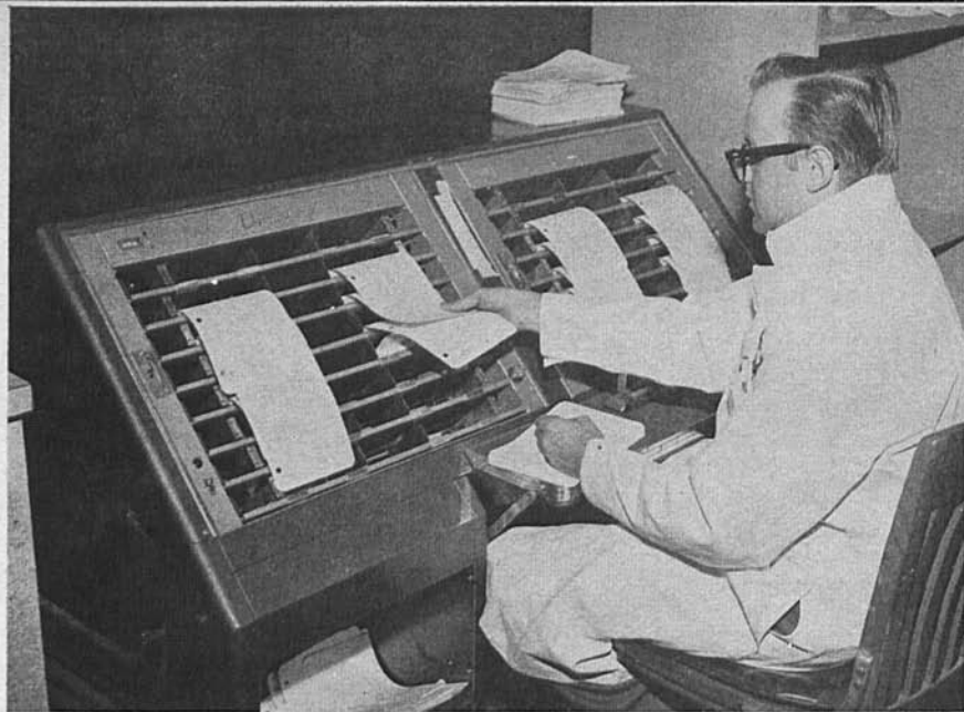
COLLATOR SAVES TIME —Arthur M. Issoglio gathers several sheets at once and in the proper sequence by use of the Thomas collator, in which an electrically-driven mechanism operated by a foot-switch pushes out single sheets from all piles of paper simultaneously.
