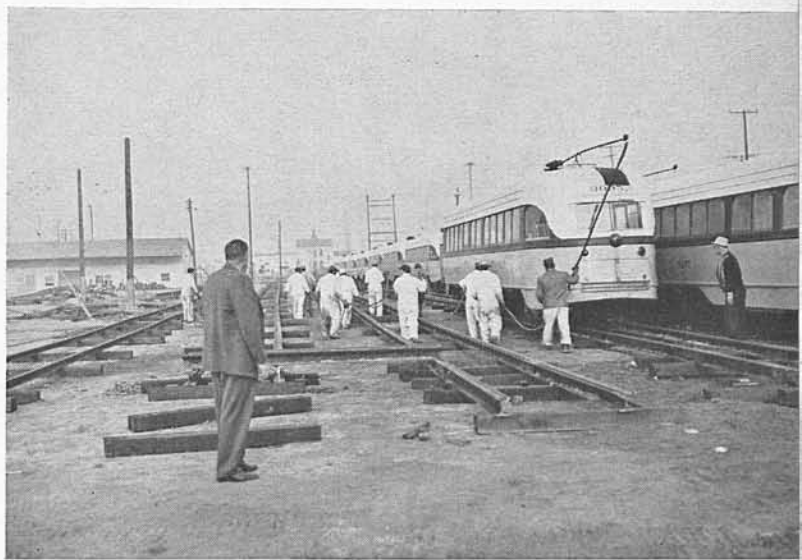
from a central switchbox to each car, where cable is hooked to trolley pole. Crew then walks along beside the car (LOWER RIGHT) with cable while a crew member, taking over car controls, moves it at a walking pace until it is bumper to bumper with the car ahead. The crew then carries the cable back and hooks it to the next car. In business suit, watching cable crew is Wheeler Ellis, Division 20 Superintendent, maintenance, now on special assignment.
