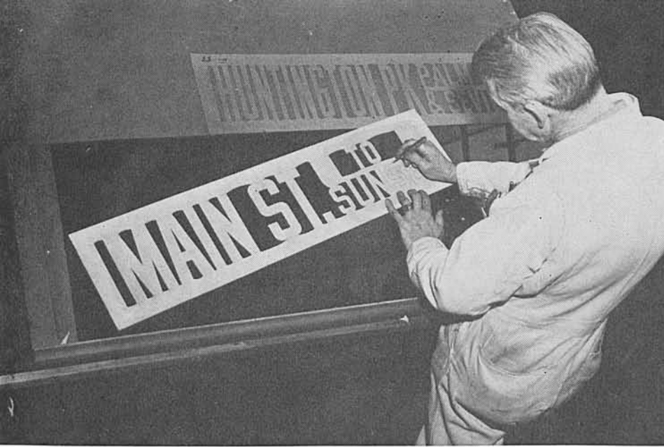
ABOVE—Many stencils involving larger letters must be cut by hand. RIGHT—"Shoe" paints many signs freehand; here's one.
