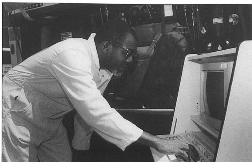
Back on the job at Division 10, Mechanic Ray Alleyne uses a Woodward Control System diagnostic computer to trouble-shoot a CNG bus engine.
