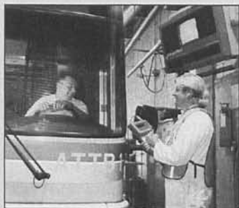
Cover Photo: MTA Mechanic Doug Creveling (r) checks the stats on the Clark ATTB during a dynamometer test at Division 10. Engineer John Gongola of Northrop Grumman, ATTB prime contractor, is at the wheel.
