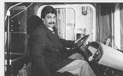
Senior MTA Safety Engineer Rufus Francis gets comfortable in the seat he designed for the ATTB. The new design should reduce operator neck and back injuries.
