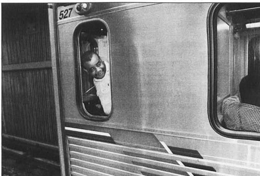
Ellis cranes out the window of his train to check that all passengers are safely on board. Red lights on each car signal doors are open; green means they're closed and he can proceed.
