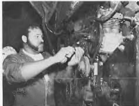
ERNEST HEGGINS prepares an engine for its diagnostic run in the first step of the refurbishing.
