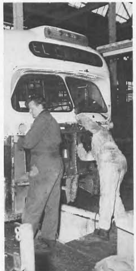
Still displaying its last destination, a Fort Worth bus receives new front body panels from MELVIN DESY (left) and OLIVER WALKER (right).
