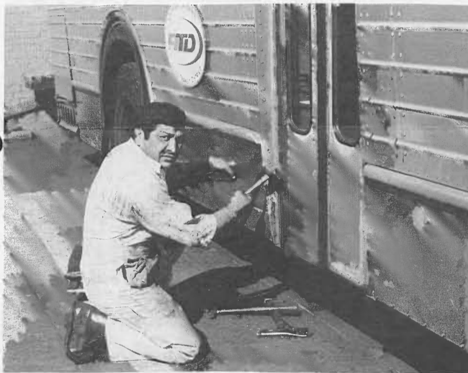
Renato Medina, a Mechanic "B" at Division 2, repairs the lower skirt panelling on a coach.
