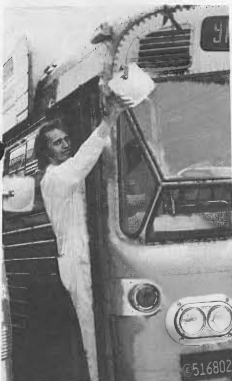
Gary Ward, a Utility "A" at Division 7, adjusts a mirror so that it won't get caught in the brushes when the coach goes through the bus washer.
