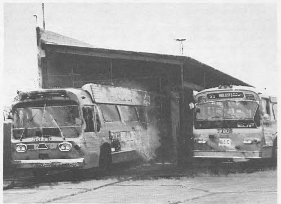
KEEPING IT CLEAN -- An RTD bus of the 5000 series gets scrubbed clean by the bus washing machine after a hard day on the road, while another bus appears to be looking on.
