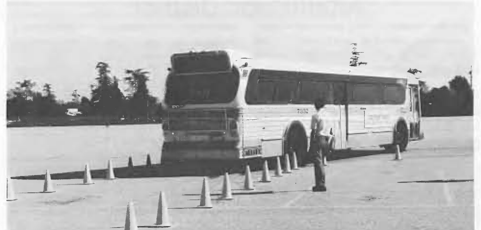
Almost unanimously, operators found that the reverse back-up movement or "bus wye" to be the most difficult maneuver. The operators had to negotiate a complete back-up in one bus length with a 4-foot clearance stopping within 3 feet of the last marker.
