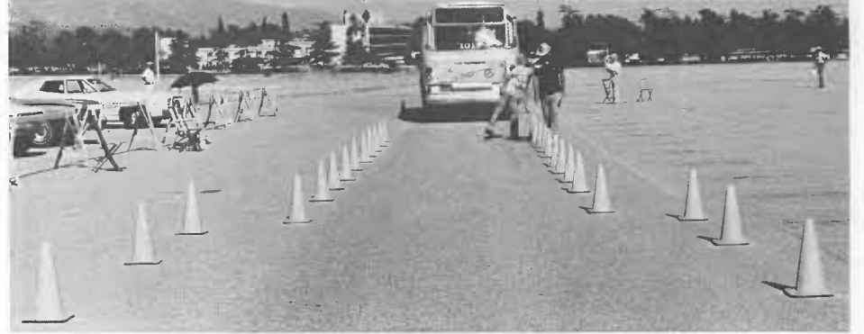
A bus goes through the "straight and narrow" the first of seven maneuvers. The maximum clearance for this was a total of 12 inches between the bright orange pylons which outlined the entire course. After this maneuver came the "serpentine," which required making three turns in four bus lengths between three pylons set 38 feet apart.
