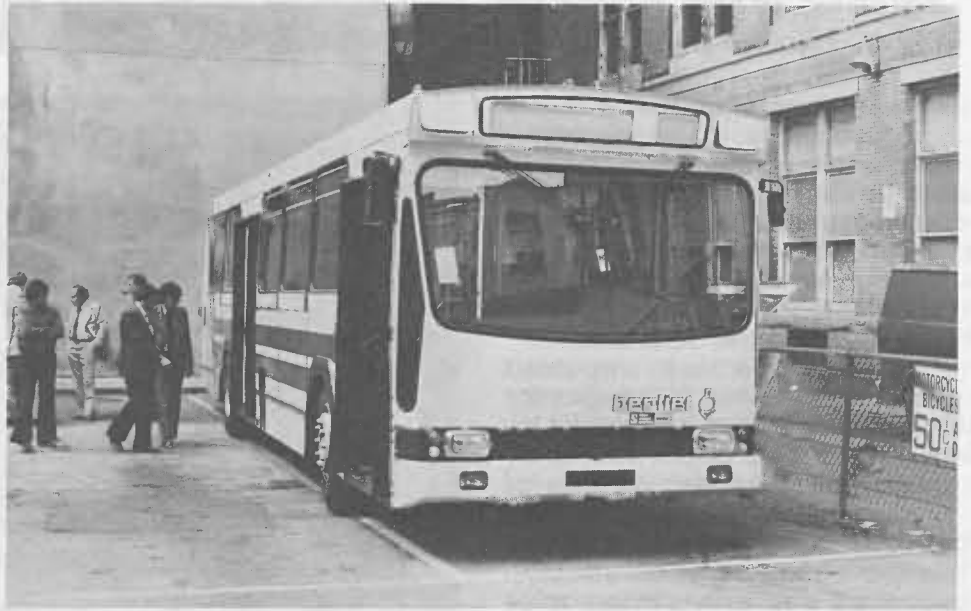
GETTING THE ONCE-OVER from District personnel is a Renault bus. The vehicle is a 41 passenger, transit type powered by a six-cylinder Renault diesel engine. It was on display outside District headquarters on April 24 for management and staff alike to inspect both its eye-catching exterior and interior.
