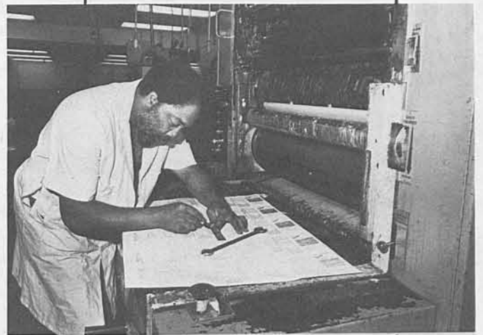
In the basement print shop at District headquarters, these layouts are transferred to metal plates, mounted on a press and used by printer Jonah Zackery to run off the timetables on large sheets of paper.
