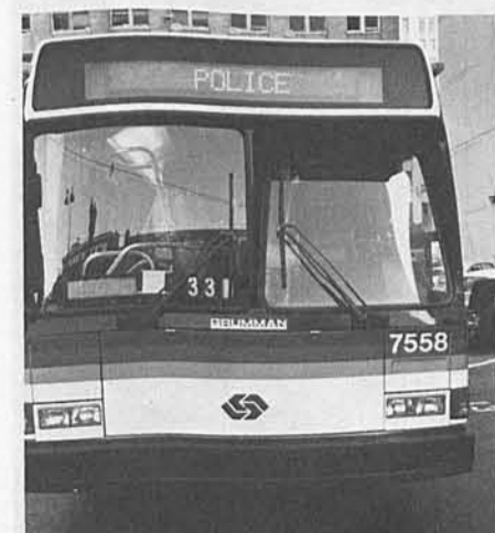
CALL SIGN — New electronic headsigns can be programmed to display a call for help.
