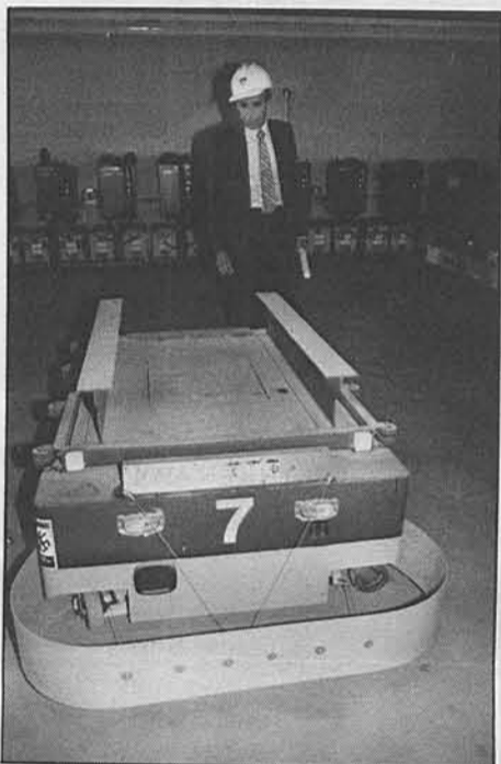
CMF Project Engineer Vasan Srinivasan looks over one of the models of robotized equipment capable of moving parts and other materiel throughout the CMF complex and known as an Automated Guided Vehicle (AGV).
