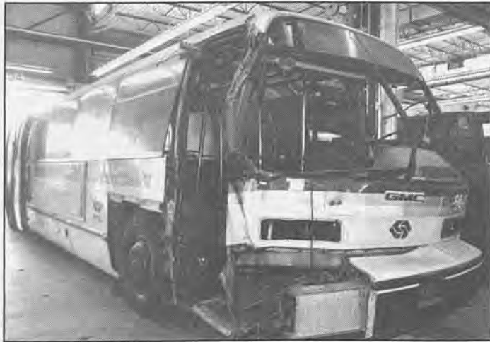
Bus #8641 suffered external right front injuries after a collision.
