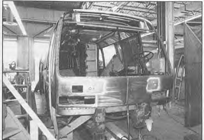
At the final stage in the Body Shop, all the panels are installed and welded. The glass will then be fitted. Made whole again, the bus is then transferred to the Mid-Life Program for updating. The last stop is the Paint Shop for that brand new look, and then its back to work for #8641.
