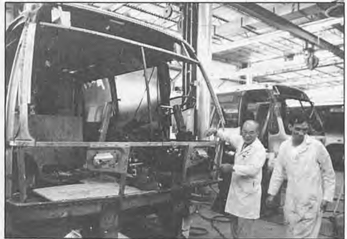
Equipment Maintenance Supervisor George Asato (left) and Mechanic A Duc Banh confer on the extent of the substructural damage.
