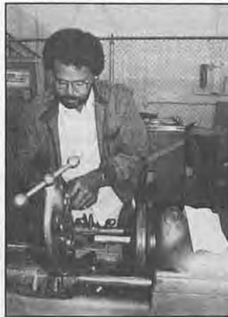
Plumber Peter Williams prepares a pipe for installation by grooving it with the requisite threads.
