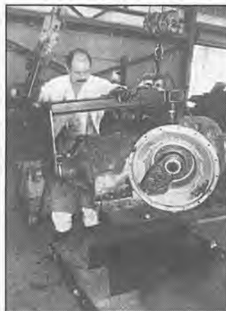
Mechanic A Tony Rodriguez lowers a V-730 transmission onto a shipping cradle and pallet.
