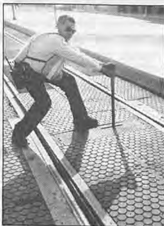
Division 1 Operator Robert Gutierrez doubles as a switchperson for the Blue Line. Using a lever, Gutierrez causes the track to switch over thereby avoiding derailment.
