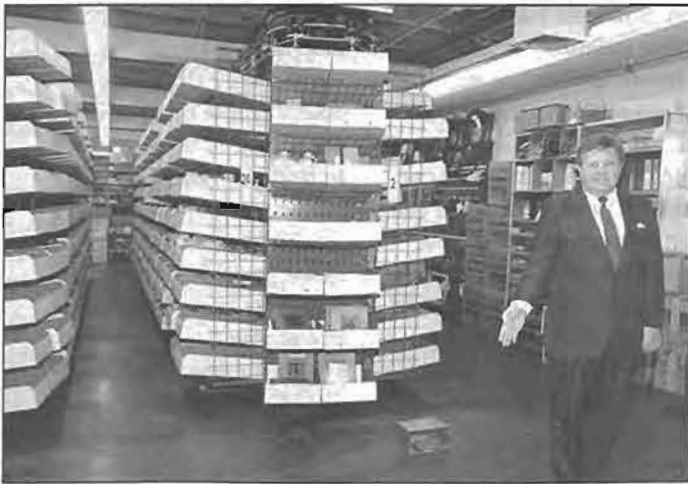
After installation of the new carousel storage and retrieval system, OCPM Assistant Director Henry Koerv points to where the conventional extended before the new was installed. The new storage system uses less space while storing more parts.
