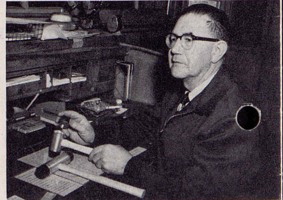
CARL L. CROSS , foreman, unit repair shop, shows new-type soft hammer with replaceable plastic faces. It lasts far longer than lead hammer, and no chips fly off.
