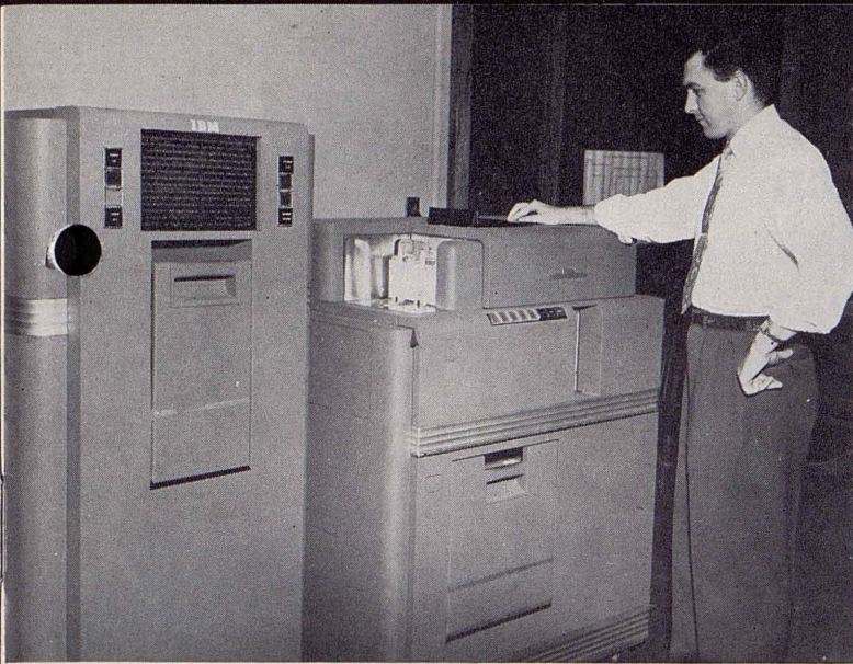
CALCULATOR —Joseph Debelak places fare box cards in this machine, which, at the rate of 100 cards a minute, subtracts beginning from end readings of cash and tokens, extends the number of tokens honored, adds token value to cash, arrives at total cash value of revenue received by first operator on fare box card, punches answers to each calculation, punches end readings for first man as begin readings for next man, etc.
