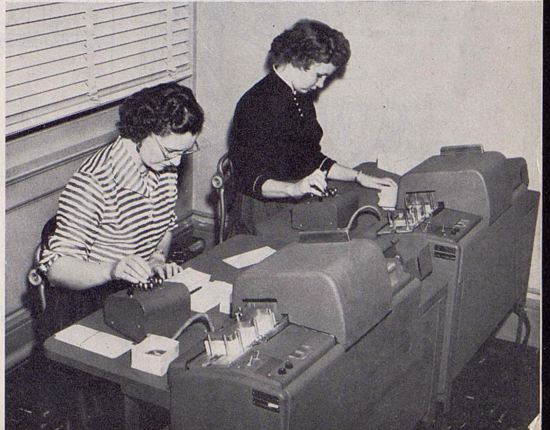
NIGHT KEYPUNCH OPERATORS Wanda Amburgey, left, and Jeanne Debelak punch and verify new cards from report as corrected by Nell, and from correct cards a revised over and short report is then run on the tabulator. More careful preparation of original cards by transportation men would eliminate much drudgery for these girls.—Daily records are kept for each man. At end of month he is charged with shortage or credited with overage.
