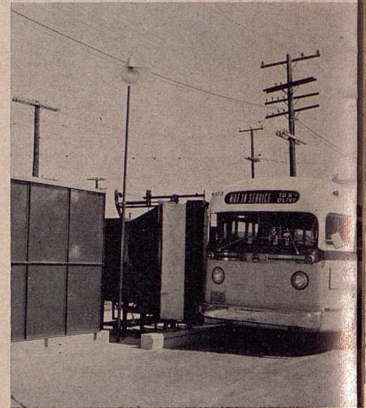
VACUUM CLEANER in operation. This one has a spray arrangement for washing papers, etc., off screen at rear of refuse container, to improve suction.
