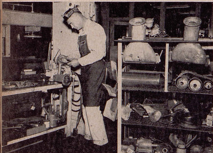
MISCELLANEOUS PARTS , such as manifolds, emergency chokes, fans, flexible couplings, etc., are overhauled by John Haberberger, shown above assembling a throttle governor.
