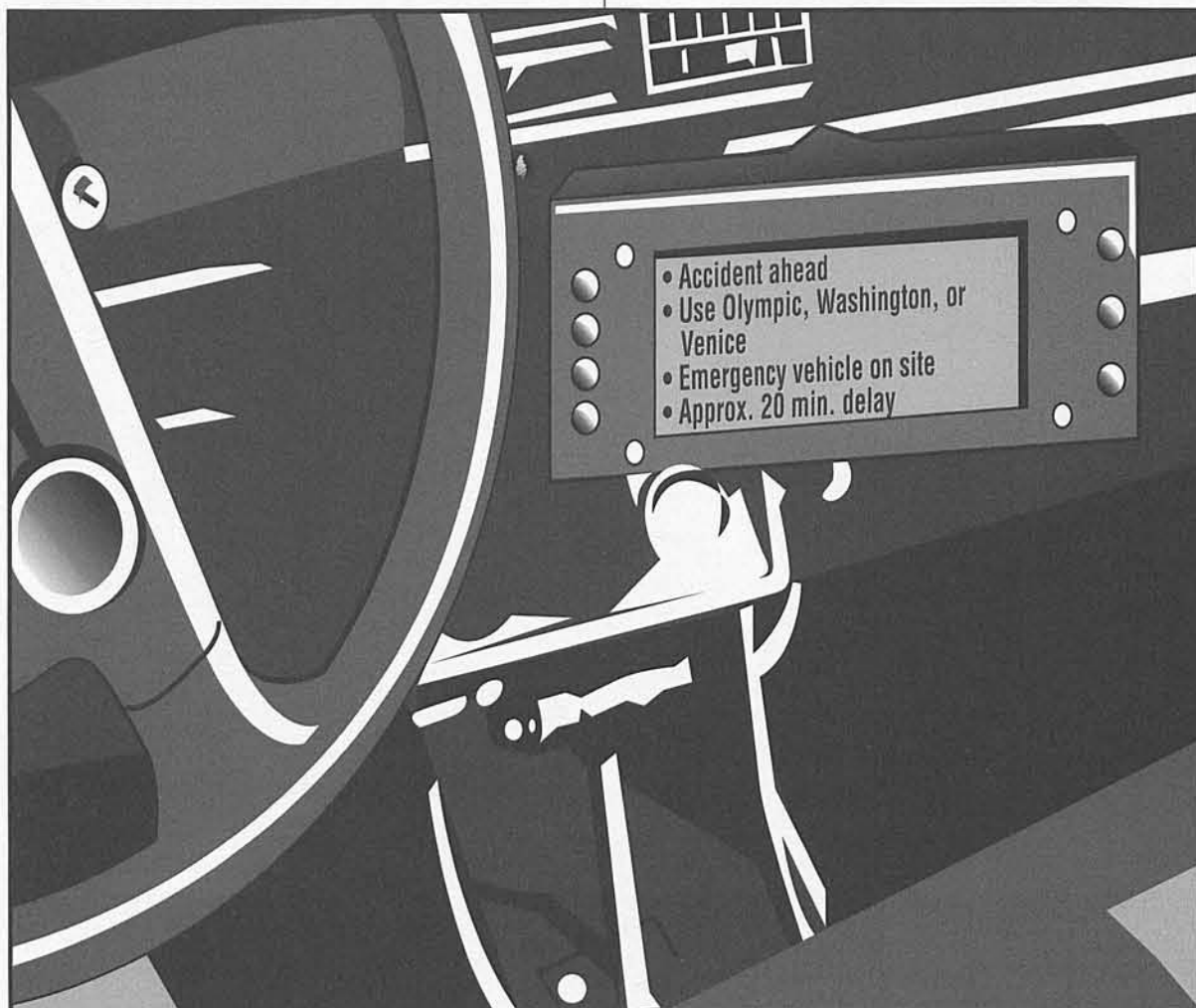
Conversational Cars —Intelligent Vehicle Highway Systems (IVHS) now being developed in Southern California, such as this interactive "inductive radio" on-board computer system, will one day enable traffic control computers and drivers to communicate instantly about road conditions and emergencies.
