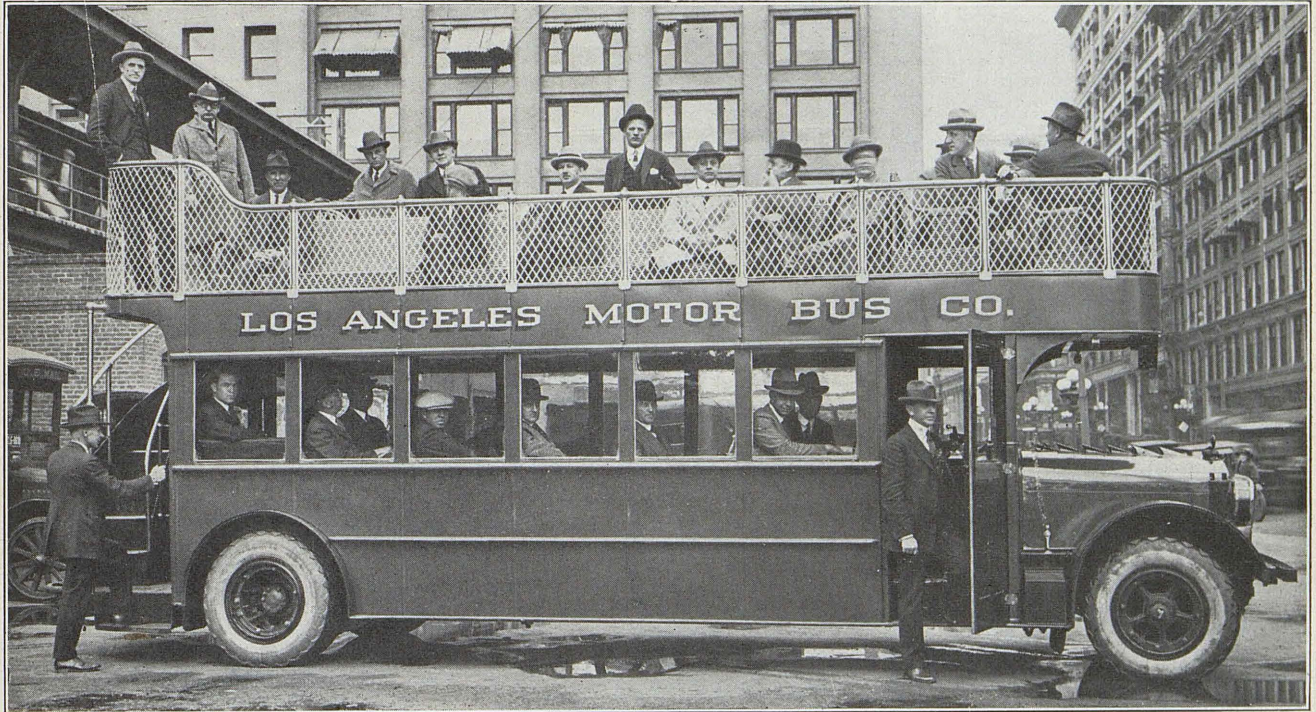
New 56-passenger Fageol bus now being tried out on the Vermont Avenue-Sunset Blvd. line of the L. A. Motorbus Company.
