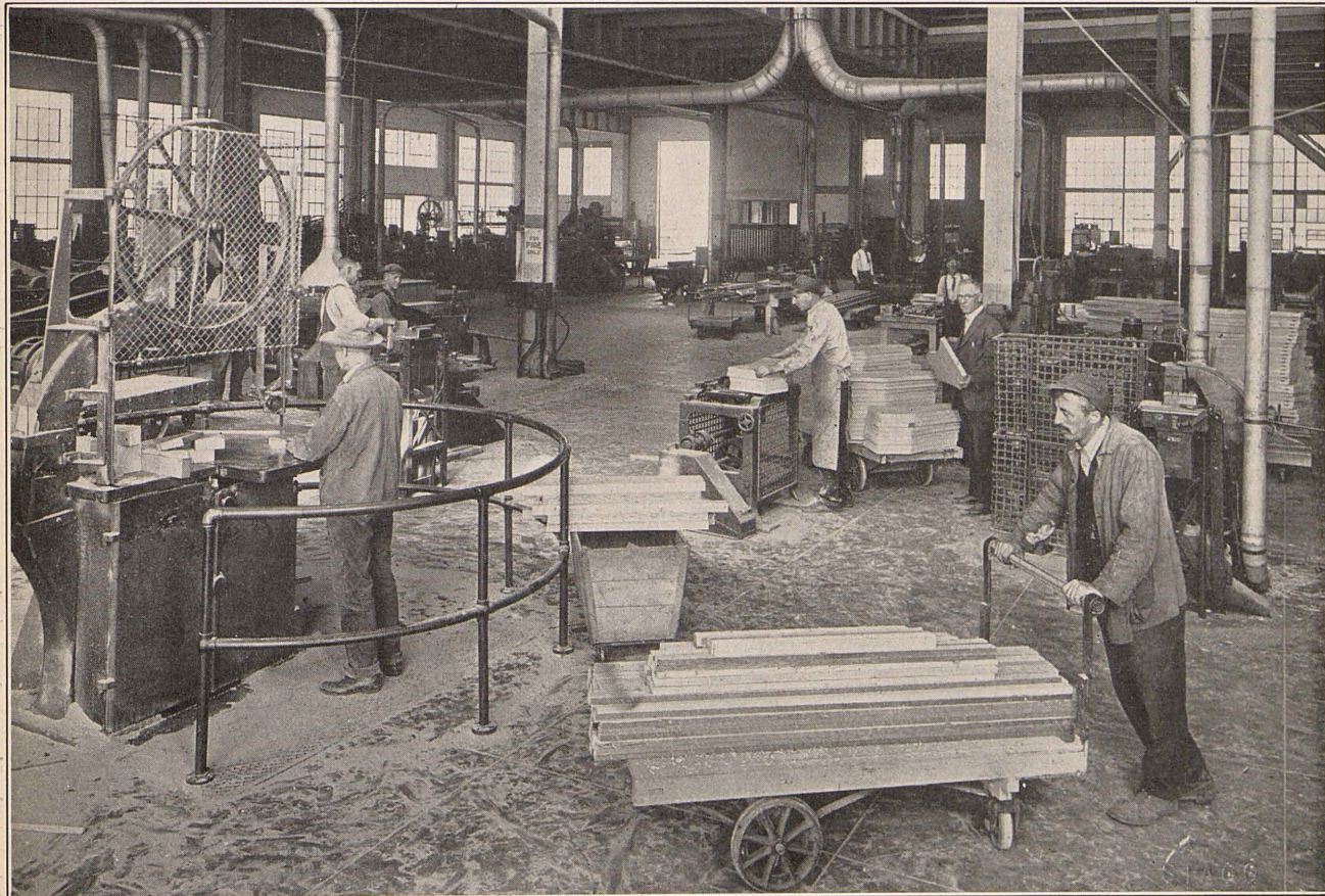
Wood mill at the Torrance shops. Note that there is no overhead shafting; each machine has its individual driving unit; danger points are screened and otherwise protected. This shop ranks with any in the United States in the matter of facilities and safety.
