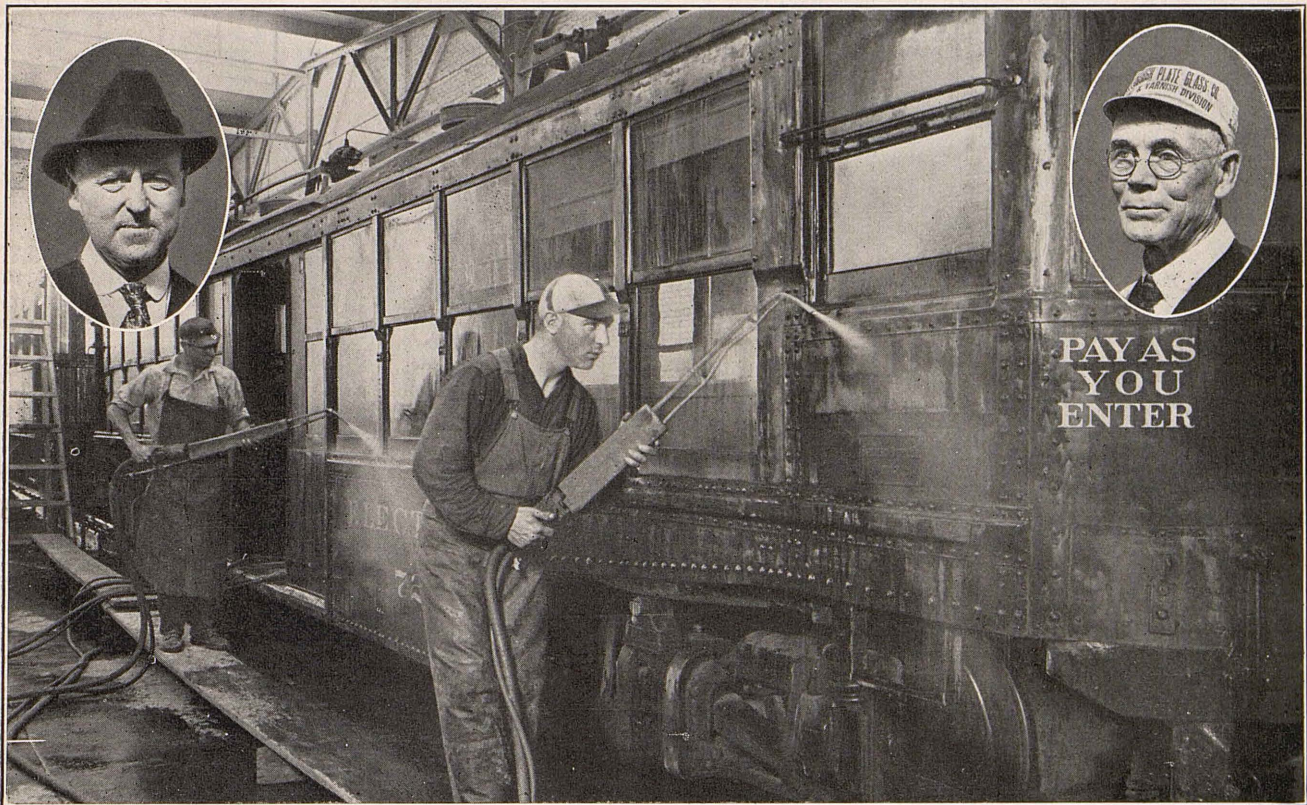
The saving of about 75% of time previously required is brought about through an improved method of cleaning equipment before painting. In inserts are E. O. Straub, left, and A. E. Fowler, who conceived the new process.
