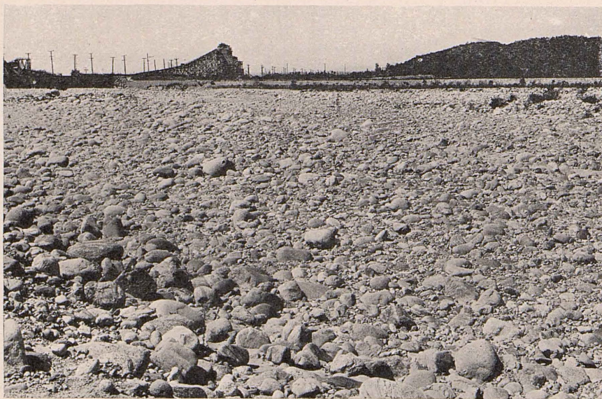
The raw material in its virgin state adjacent to a Union Rock Company plant. These river washes are worked to an average depth of fifty feet.
