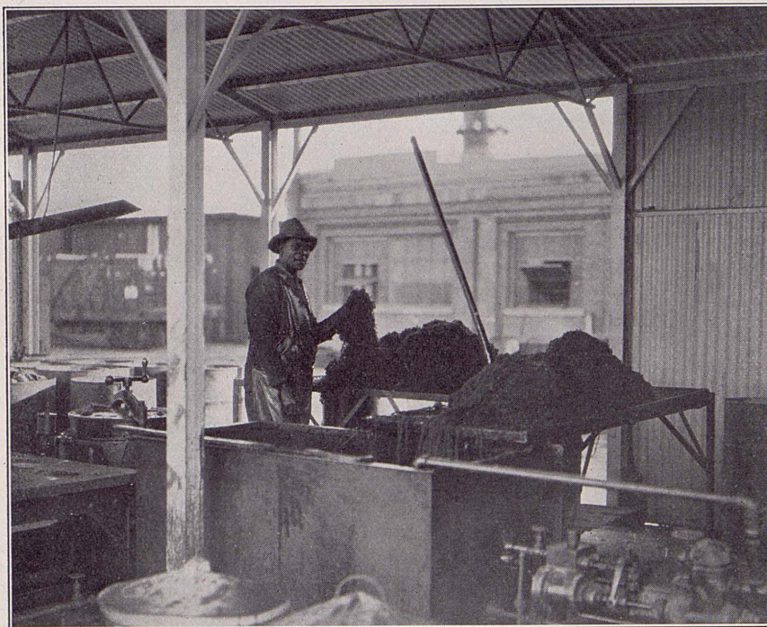
Used waste and oil are restored to usefulness in salvage plant in our Torrance Shops, netting a considerable saving each year.
